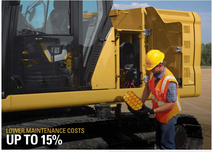
With extended and more synchronized maintenance intervals, you get more done at a lower cost compared to the 320D2. Consolidated filter locations make service faster. Hydraulic, air and fuel tank filters have increased capacity and longer life.
