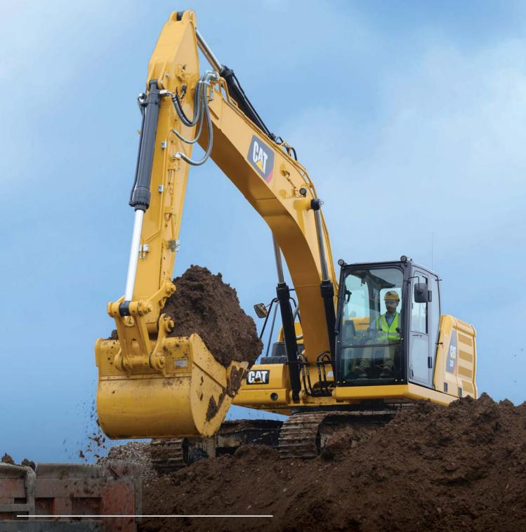
Engine Power Operating Weight 117 kW (157 hp) 22 000 kg (48,500 lbs)
